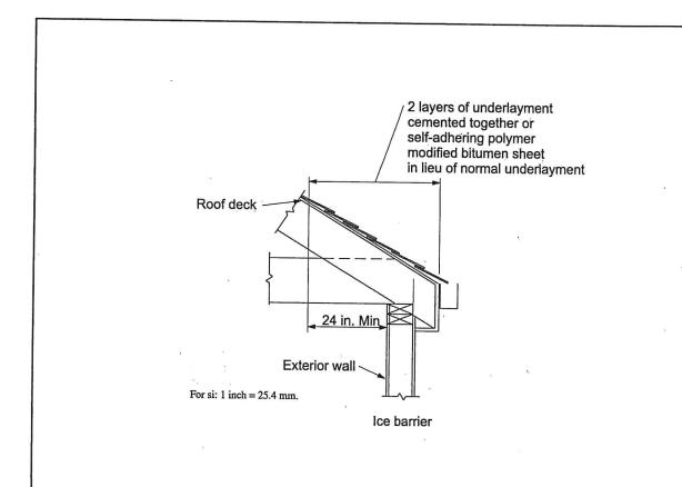
The requirement for an ice barrier is not limited to the application of asphalt shingles. Similar requirements are applicable to roof coverings of mineral-surfaced roll roofing, slate and slate-type shingles, wood shingles and wood shakes.
