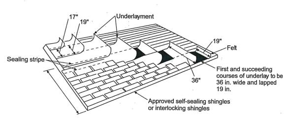
Note: In areas where there has been a history of ice forming along the eaves causing a backup of water, special methods, rather than normal underlayment, shall extend up from eaves for enough to overlie a point 24 in. inside the wall line of the building.
